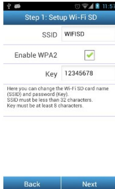
Step1. Modify the Wi-Fi SD SSID and Key or tap **Next** to skip this step
